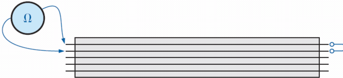
FIG. 3.30 Identifying the leads of a multilead cable.
