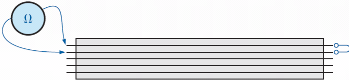
FIG. 3.30 Identifying the leads of a multilead cable.
